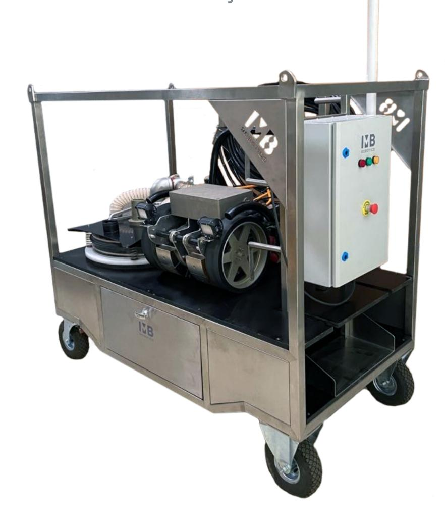
The transport system is designed to carry all the kits and addons with its multi purpose frame to mount control cabinet and wind power cables or hose.
