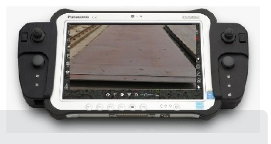
The AWC is built on rugged 8" android tablet. And it has all-weather IP65 dust and water-resistant design. This enables the AWC to work even in the most restrictive conditions. The AWC is a universal and radio agnostic ground control station. It is a well-proven, secure, and reliable solution which is easily adaptable to your hardware and software requirements. You can easily control all your equipments from one system.
