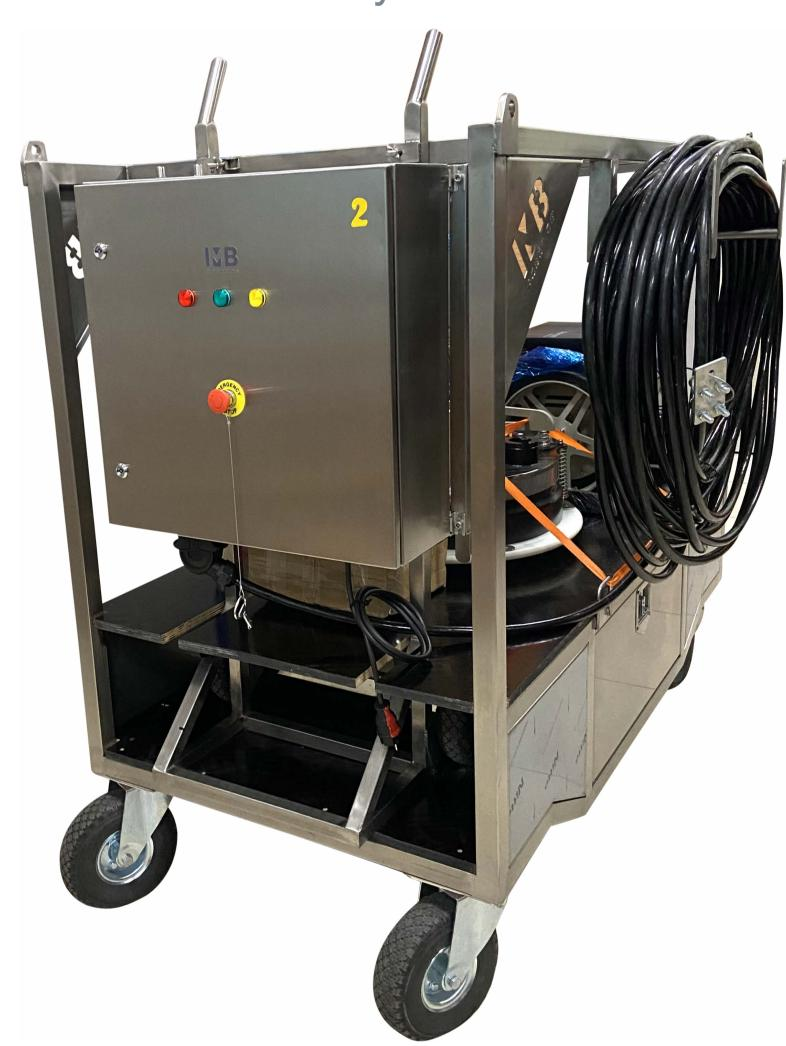
The transport system is designed to carry all the kits and addons with its multi purpose frame to mount control cabinet and wind power cables or hose.
